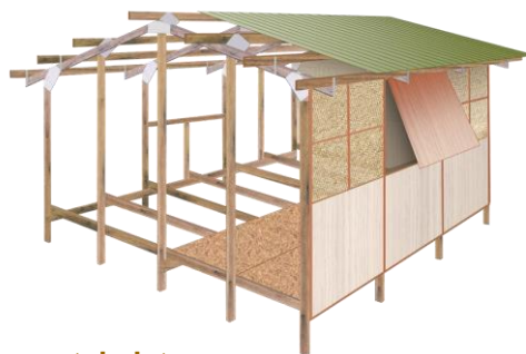
Timber with scrap metal plates
